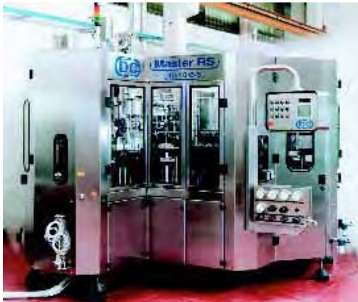
Rinser-filler-capper: Sympak Master RS 40-head rinser-filler with twin 8-head cappers
