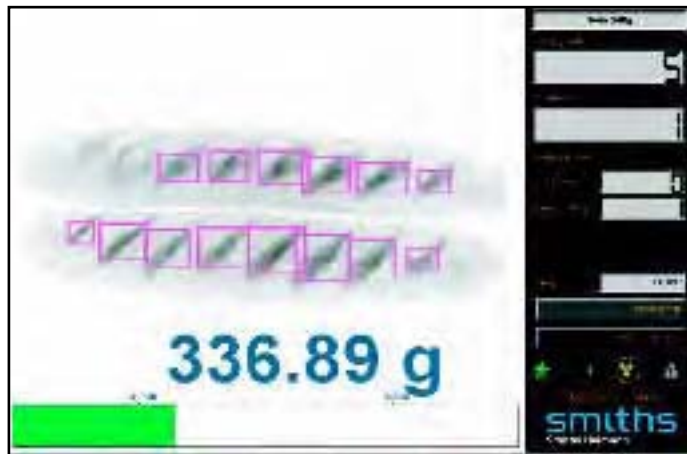
Monitoring garlic bread: Weight is within tolerance, there are no contaminants, but two of the 16 butter portions are missing
