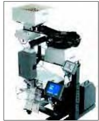
Counting machine: AccuCount 200 mounted on an Autobag bagger
