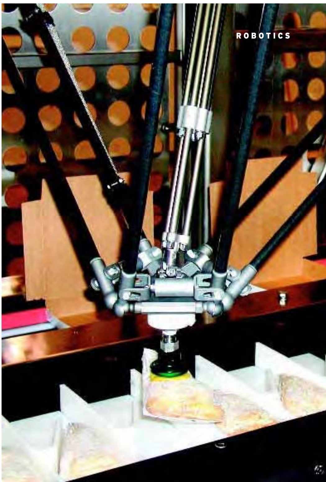
High speed pizza packing: Part of a Bradman Lake cartoning line handling 800 portions a minute
