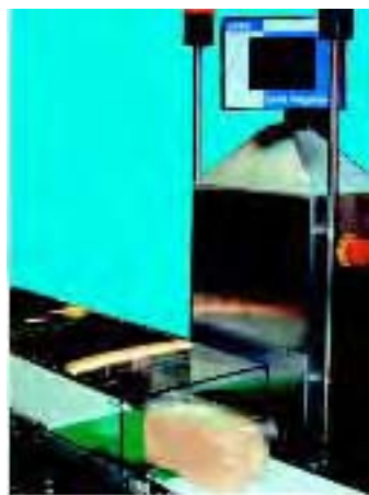
Combination: Weighchek checkweigher and metal detector
