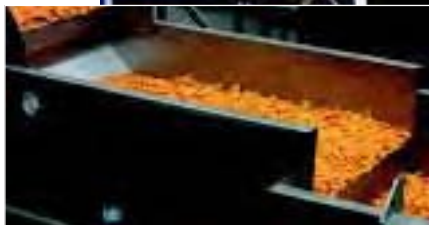
Snack flavouring line: The flavouring drum (above) is fed via a Weighwright vibratory weighing conveyor (left) which provides mass flow measurement for the dosing system
