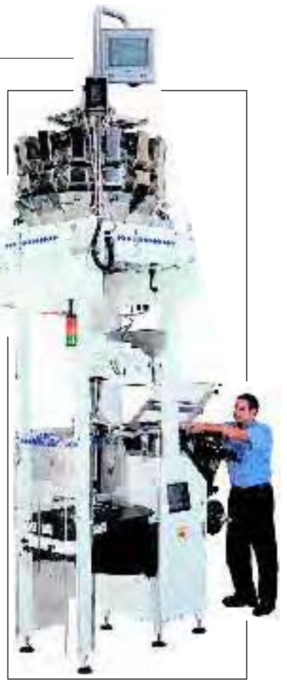
Raising output: Robag 3fx bagger with TNA Delta 1 multihead weigher
