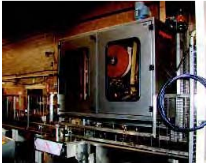
Keg labeller: The Logopak 906 TK labeller installed at Bulmer's Cider
