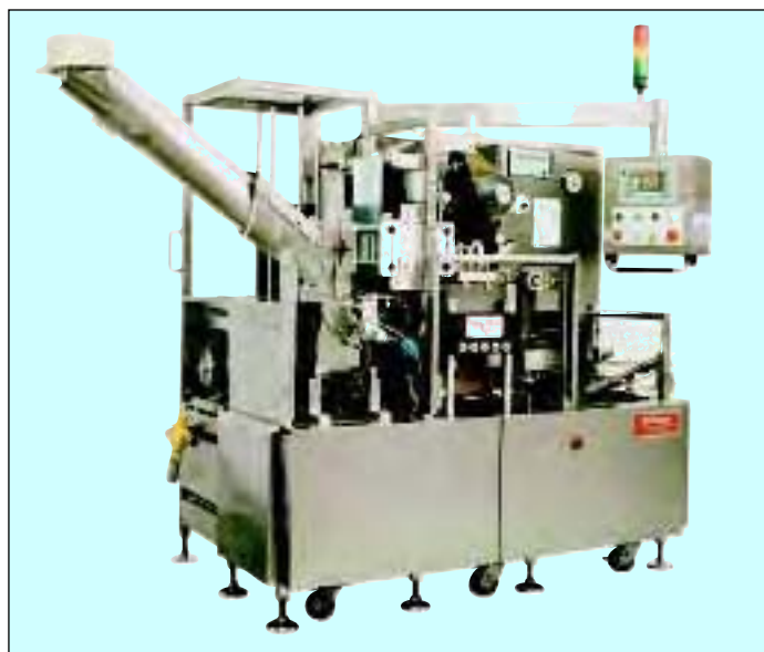
Compact ready meals line: Raque system gives speed up to 35 cycles a minute
