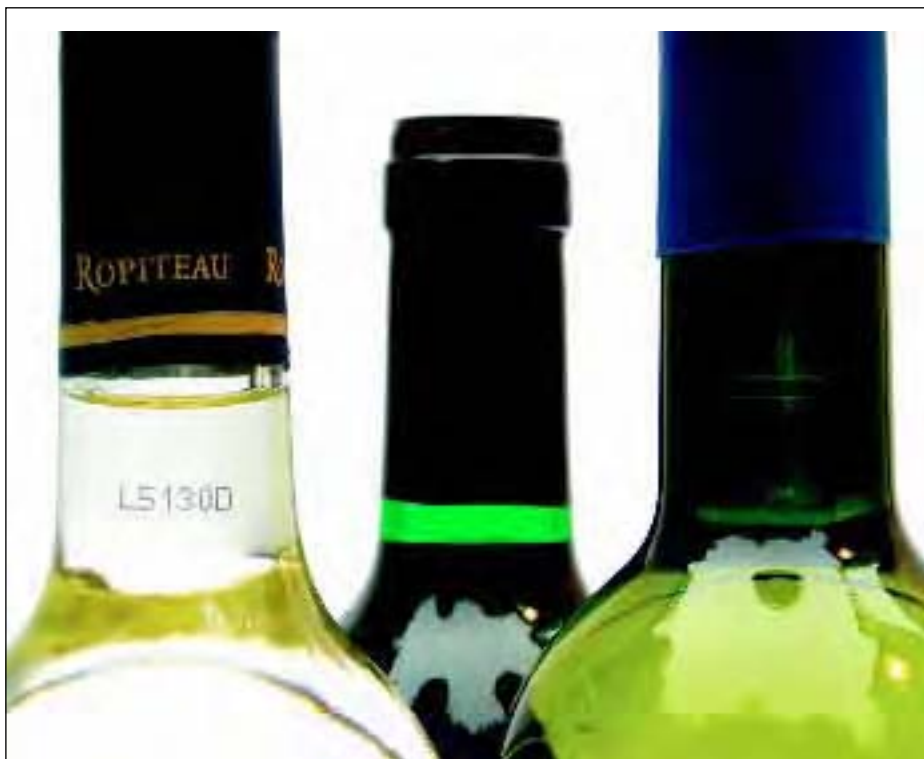
Lot number coding: Waverley TBS uses small character ink jet coders from Imaje
