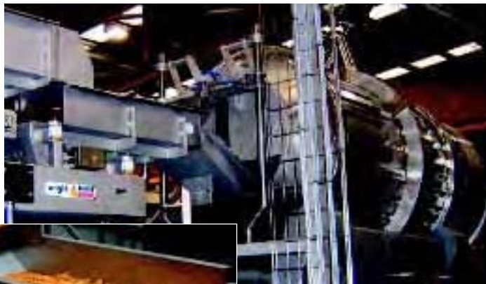
Snack flavouring line: The flavouring drum (above) is fed via a Weighwright vibratory weighing conveyor (left) which provides mass flow measurement for the dosing system
