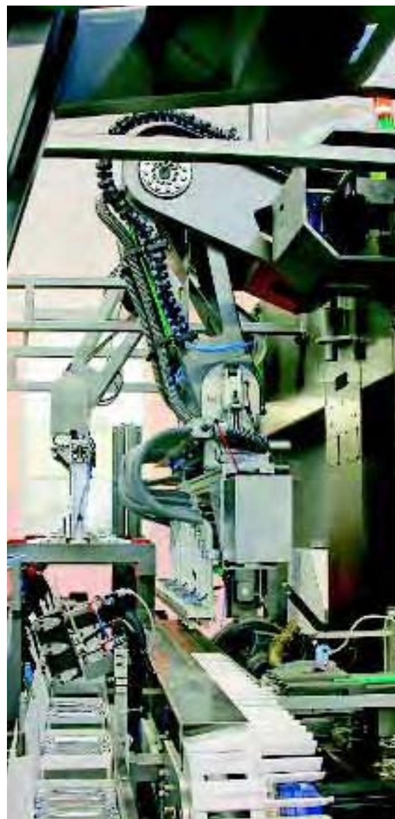
Single controller: Elau PacDrive runs the host machine and the robots used for loading
