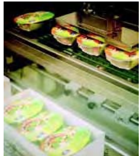
Loading transit packs: Ishida FPS system
