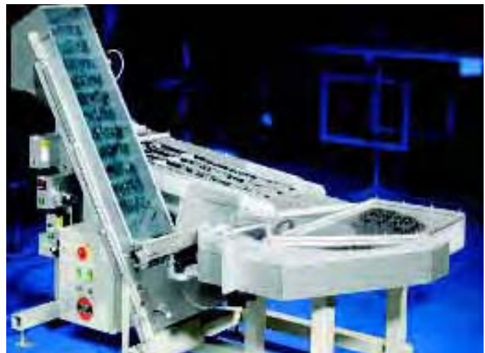
High speed: Unscrambler delivers over 2000 items a minute from eight lanes
