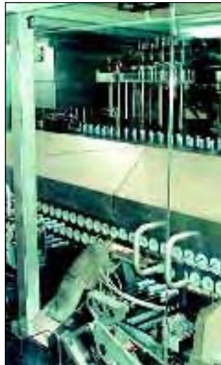
TFS 80-6 tube filler from IWKA is capable of 500 a minute. 31
