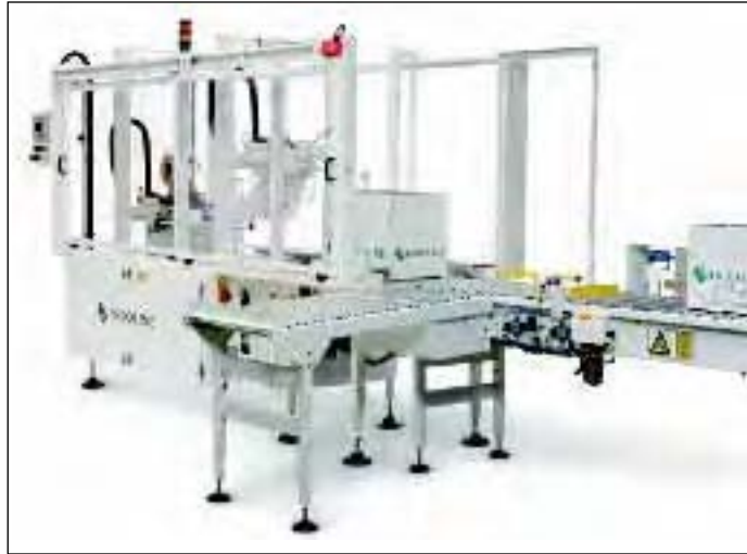
Faster operation: Endoline 734 taper identifies case size via scanners
