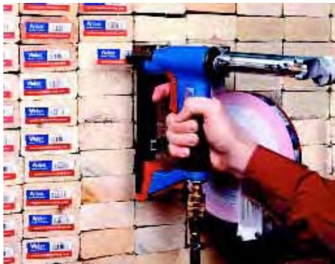
Bar coding for timber: FasTagger stapling gun from Weber
