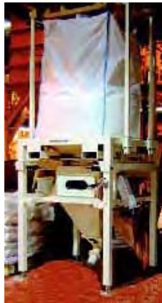
FIBC discharger: Top section with bag is lifted into place by a fork truck
