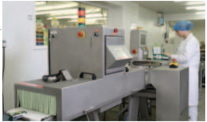
Searching for contaminants: Cintex Sentry XR low cost X-ray machine
