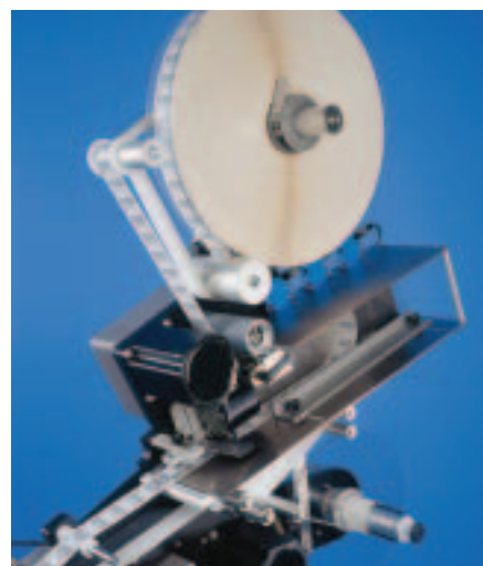
Pagomat 6/3: Buffer label loop is tensioned by air
