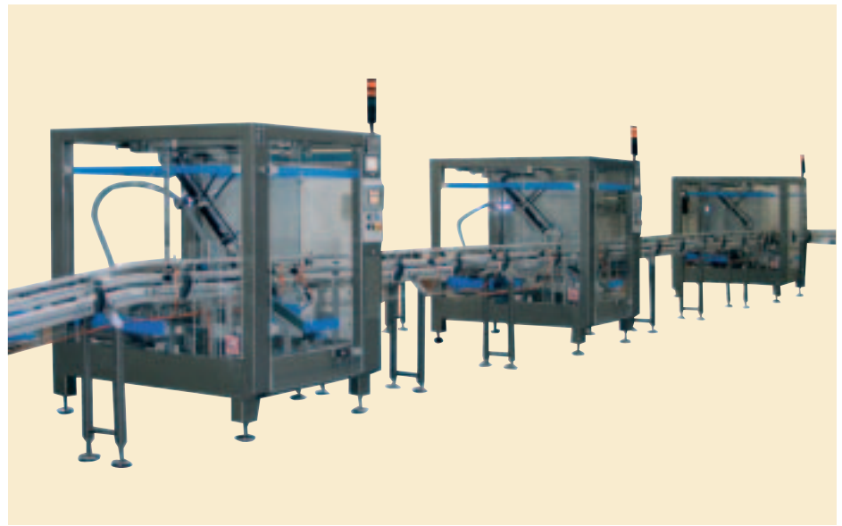
Robotic trio: Cama system loads three components of various cake mixes
