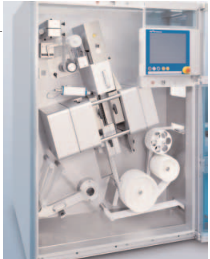
Forming station: Reciprocating carriage carries the heating panel and tools
