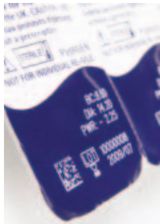
Domino ink jet system for late stage customisation of pharmaceuticals. 16
