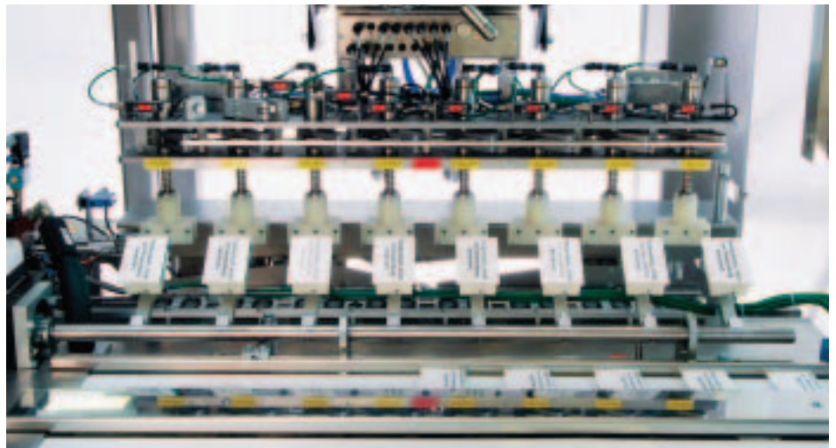
Wallet loader: Tablet blisters are glued into carton strips by the Schubert TLM-F2 line
