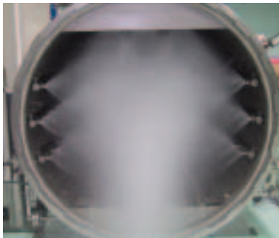
Steam and atomised water: Surdry units are said to give even heating
