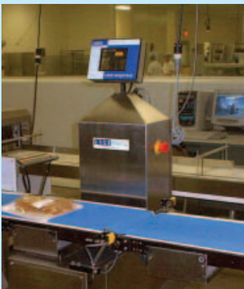
Final check: Lock WeighChek checkweigher is combined electronically with a metal detector
