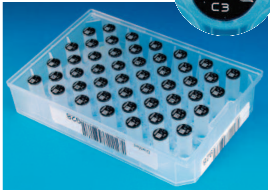
Each well identified: Cognex/Technifor system codes and verifies each well of a tray of samples
