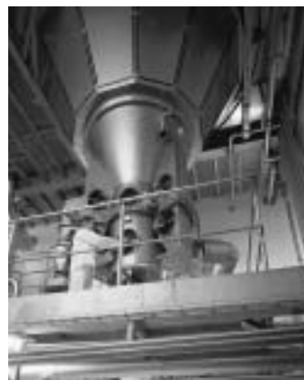
Spray drying: Niro machine provides dust free agglomerated powders
