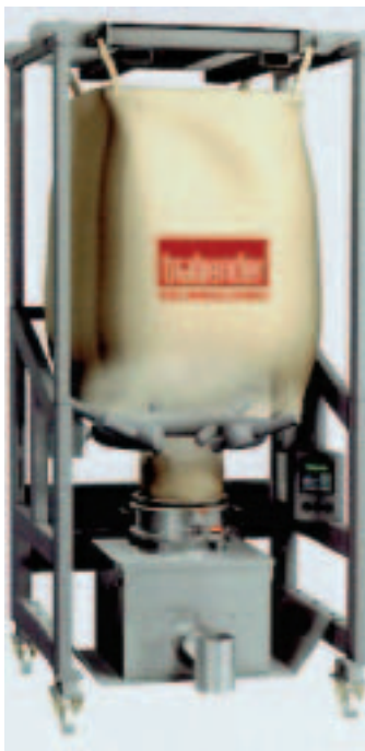
Improved discharge: Brabender system uses a "massaging ring"
