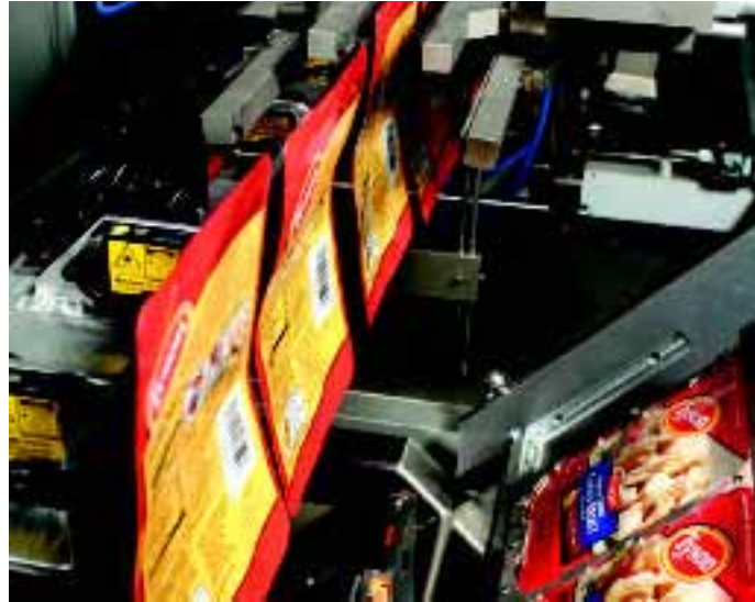
Loading by robotics: Pre-made pouches are fed to the walking beam
