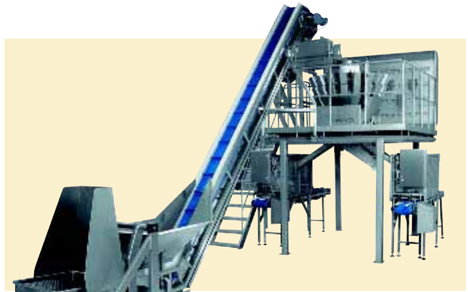
Feeding two lines: Adams Pork Products is using an 18-head Bilwinco combination weigher
