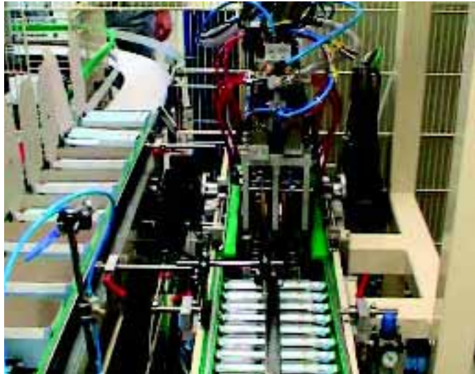
Compact system: Vepatec top loading station for confectionery bars
