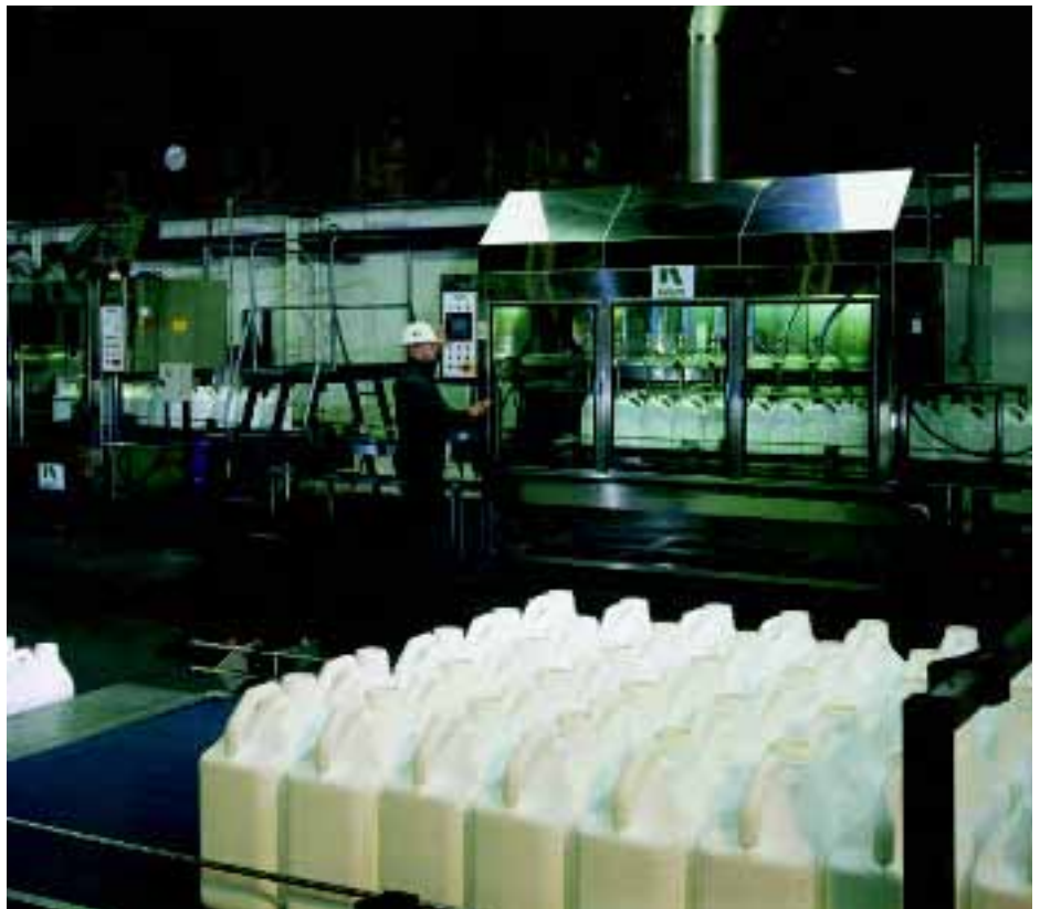
Flowmeter filling: The heart of the Nufarm line is an eight head Masterfil machine
