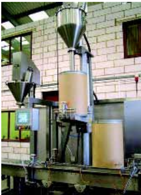
Bottom up filling: All-Fill system handles 75kg drums of micro-cellulose powder
