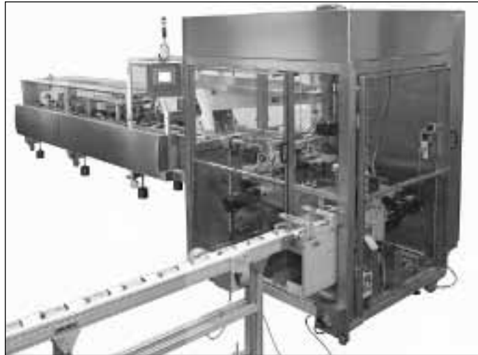
Lower cost: Bradman Lake end-load cartoner with racetrack collator
