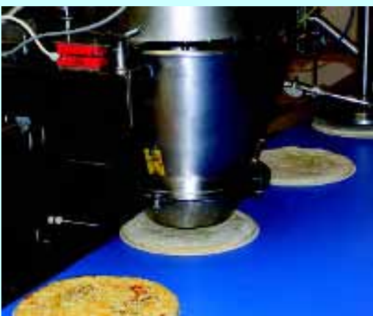
Placing pizza topping: Turbo systems has supplied Anaka Foods with this D150 depositor
