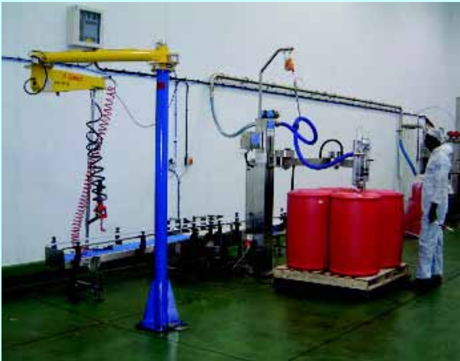
Filling a variety of containers: Weightron Bilanciai weigh-fill line handles caramel for the Healy Group
