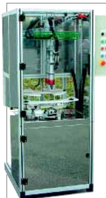
Versatile capping: Cap Coder CC560 handles a range of bottles and caps
