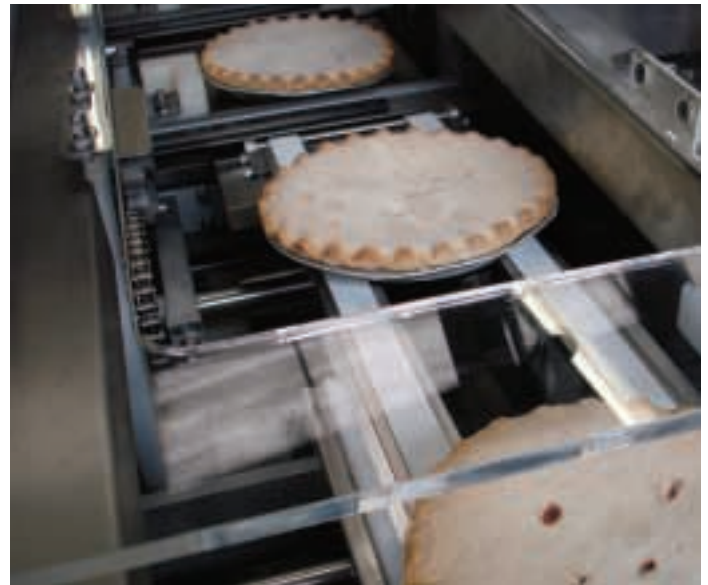
End loading: Pies are fed into the pushers of the Freemantle cartoner
