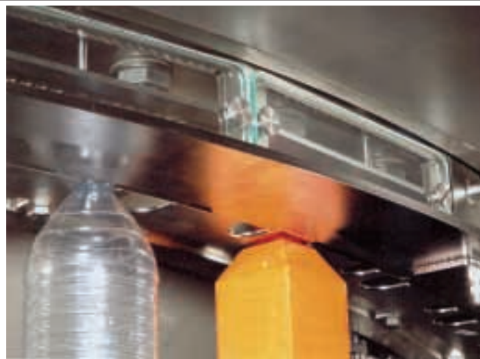
Flexibility: Neck ring isolator allows a variety of container shapes to be handled
