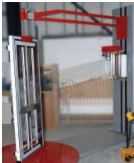
Transit pack: Stretchwrap protection for windows
