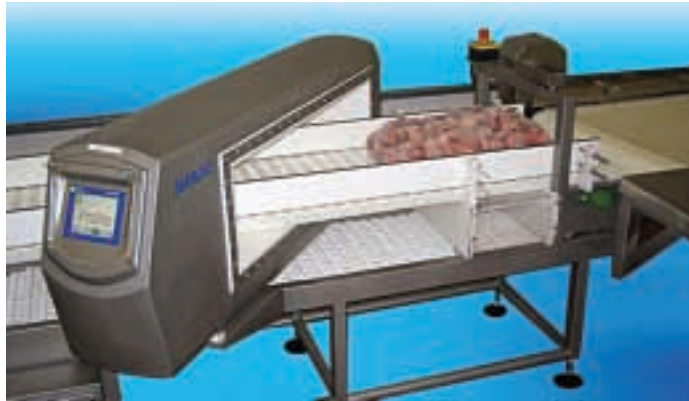
Searching at different angles: One of three heads on the Mettler-Toledo system
