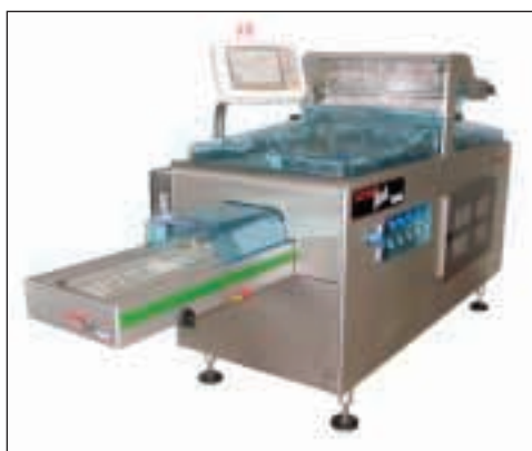
Stretchwrap MAP: Atmopack wraps 40 trays a minute
