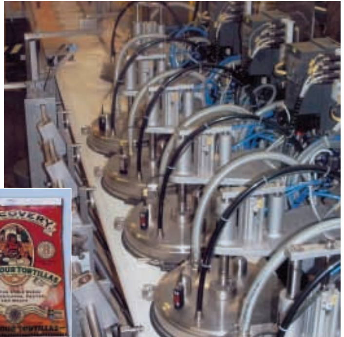
Extra shelf life: Air is extracted from tortillas by the Ilapak VacMap machine immediately prior to wrapping
