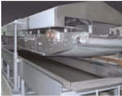
Food processing: TNA nut and legume fryer is said to use less oil
