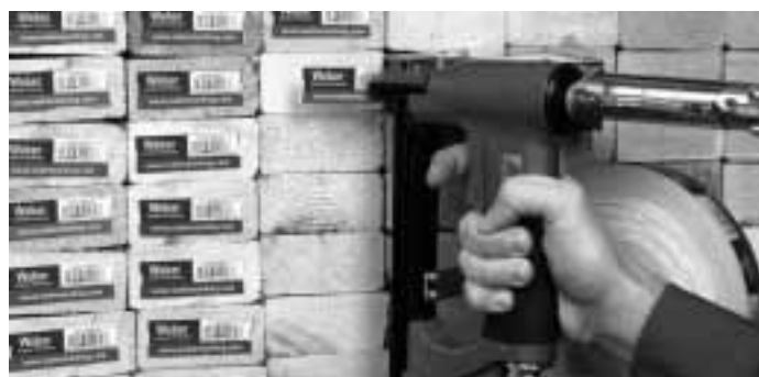
Faster coding: Weber FasTagger can apply 100 labels a minute
