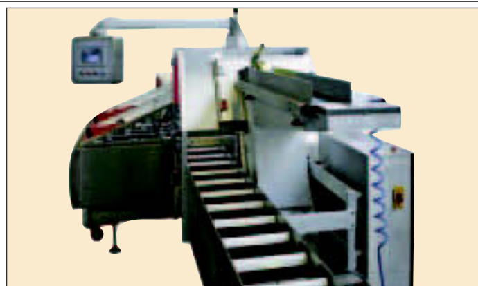
Lower cost: Bradman Lake SL903 automatic end-load cartoner
