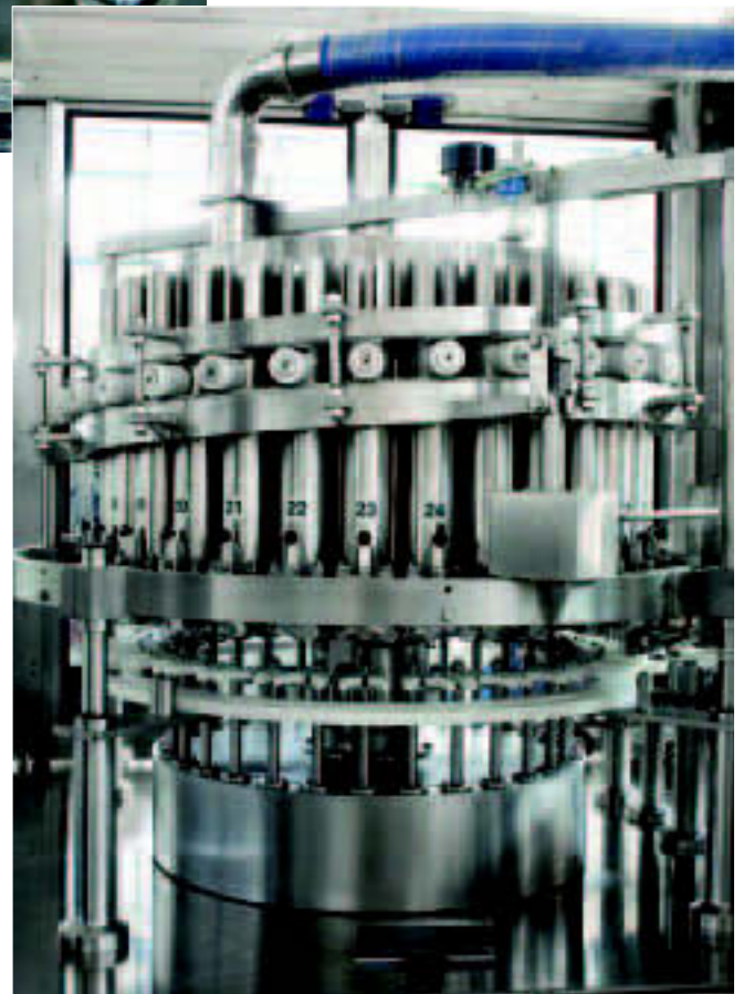
No sizeparts: Thirty-head piston filler from Planet Flowline
