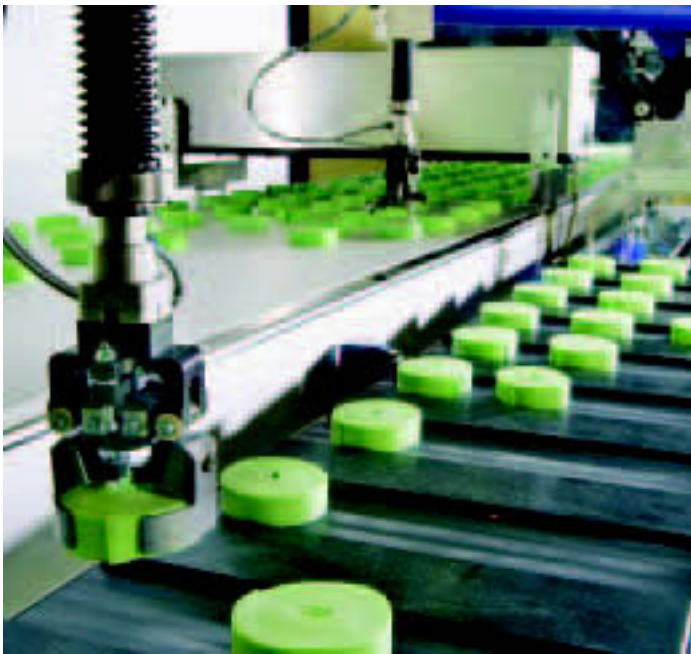
Handling bubble gum: Robots transfer rolls of gum onto product carriers
