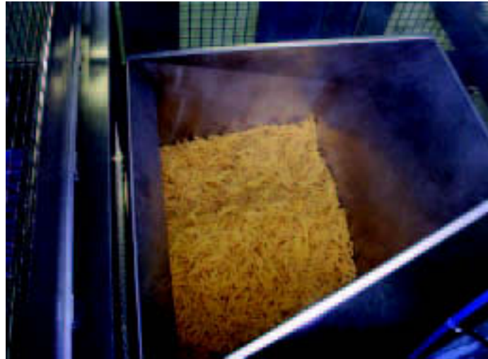
Continuous cooking: Vortex S cook, quench and chill system
