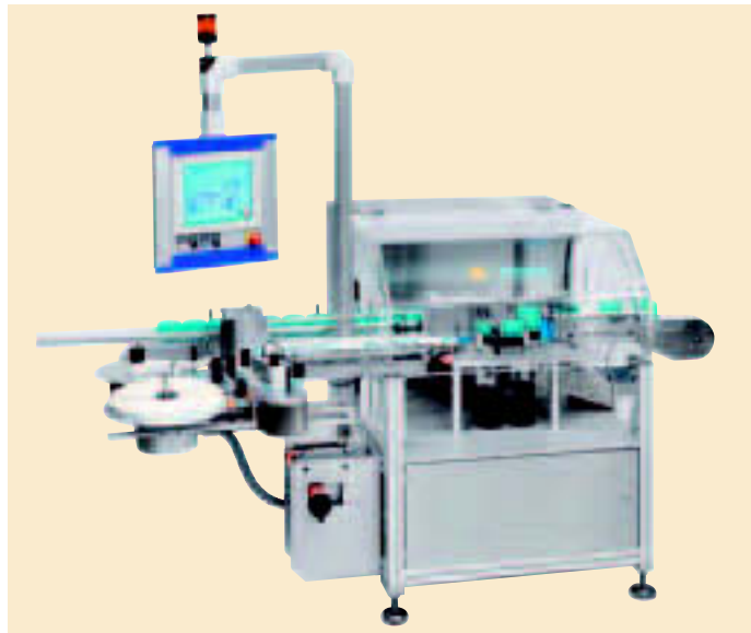
Herma UK: Demonstrating the 132M wraparound labeller
