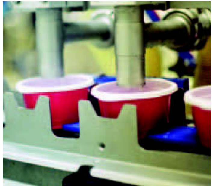
Avoiding seal contamination: Ishida walking beam transport for soup pots
