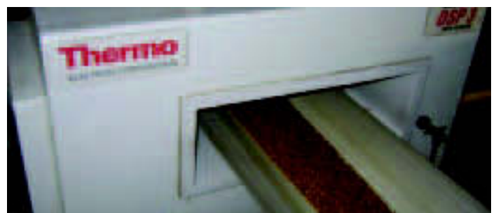
Monitoring grain: DSP3 machine handles up to 12 tonnes an hour
