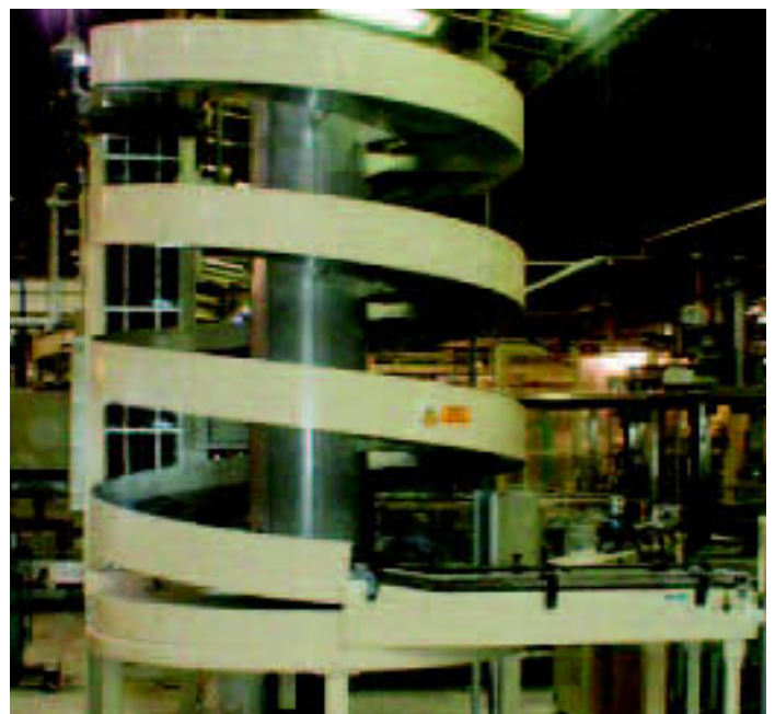
Astec Conveyors: Spiral conveyor can also act as a buffer store
