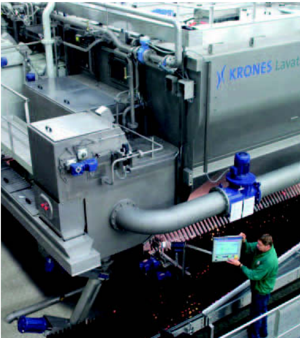
Reduced costs: Dutch brewer Bavaria has installed the first Krones Lavatec KD 2005 double ended washer
