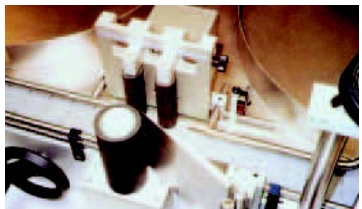
Atwell Labellers: Tri-Roller applicator for cylindrical products
