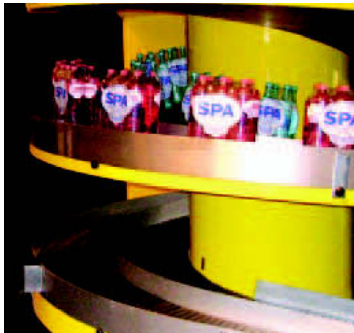
Conveyor Systems: New twin lane Spiralveyor
