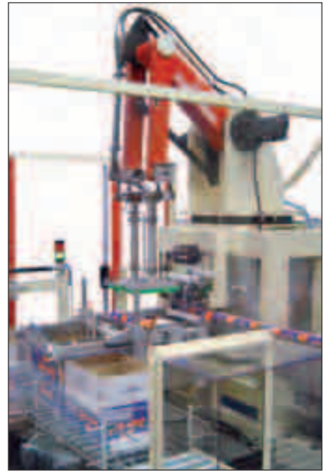
Upgraded line: Sewtec case-packing system at United Biscuits, Manchester
