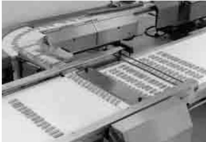
Distribution system: Autowrappers' ADS aligns and feeds bars for wrapping
