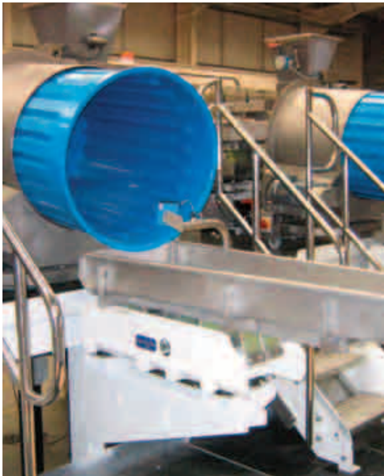
Individual drums: One flavouring drum per line ensures product consistency
