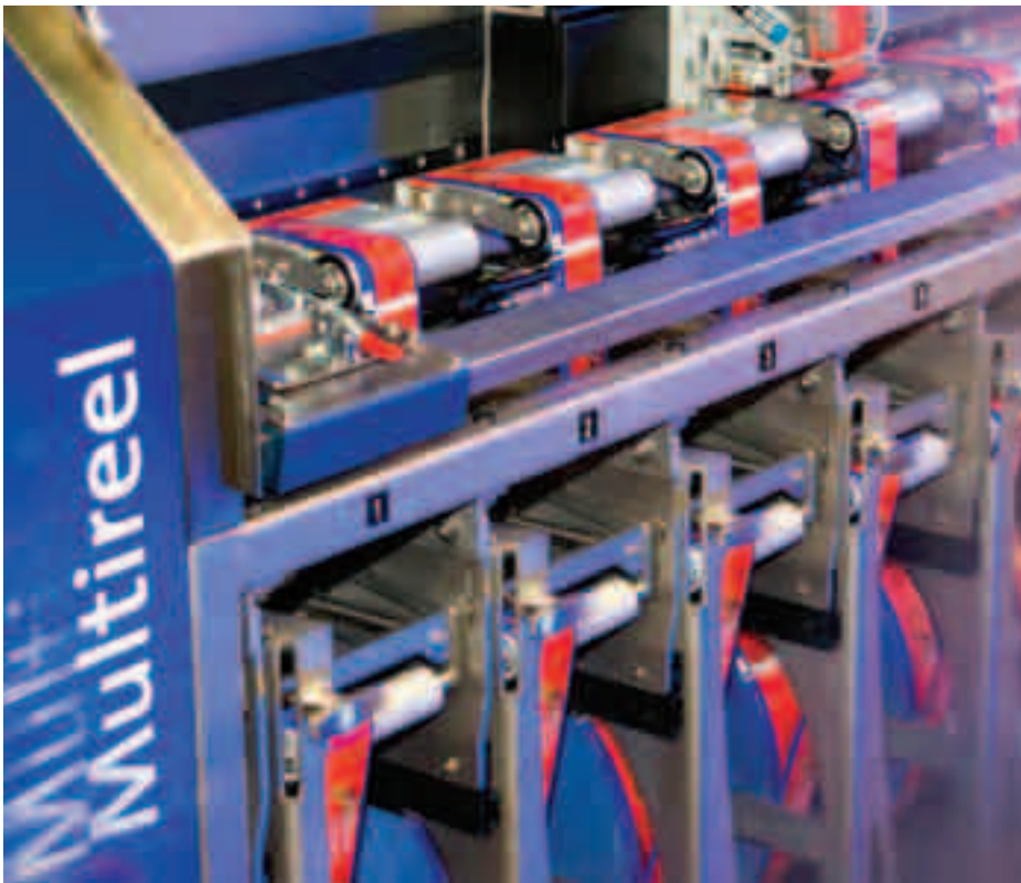
Uninterrupted labelling: New eight reel magazine allows Krones Controll labeller to run for four hours
