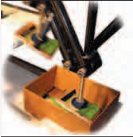
Case-packing flexibility: Fallas robot with Elau controls can load a variety of layer patterns
