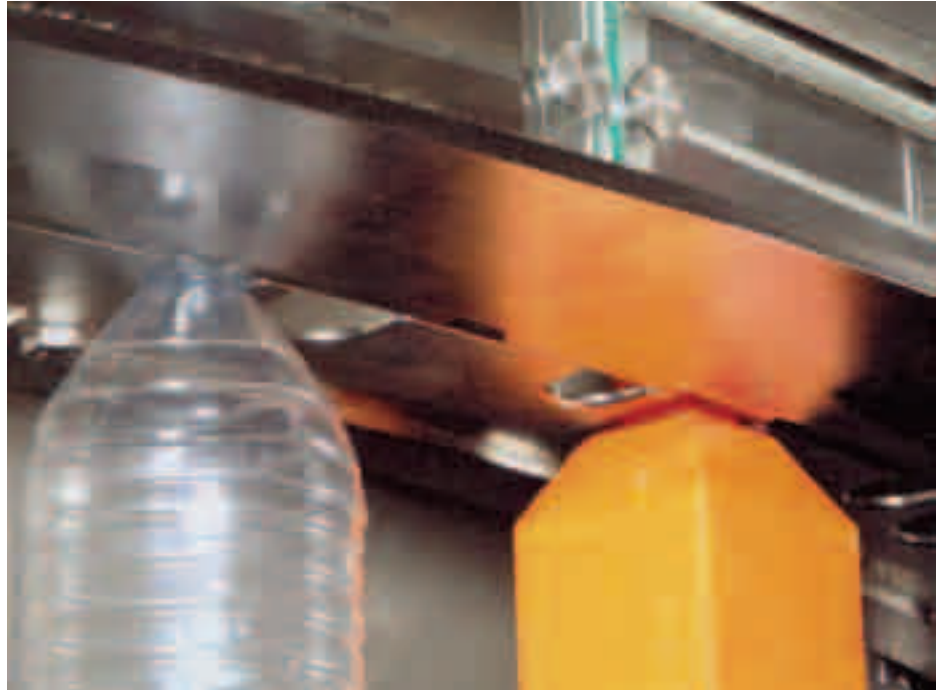
Aseptic flexibility: Neck ring isolator from KHS allows a variety of container shapes to be handled
