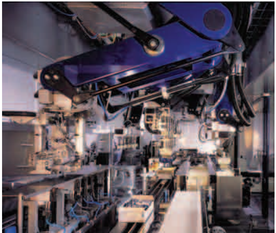
Packing filters: Brita has bought its third Schubert system to pack four different types of filters into cartons
