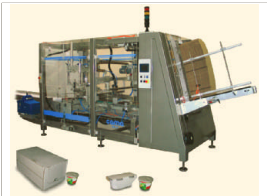
Wraparound case-packing: Cama machine handles multipacked pots at 13-26 cases a minute
