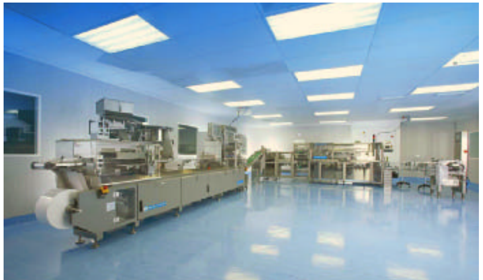
Latest line: Brecon Pharmaceuticals' new Noack 623 blister packer and Promatic 4200 cartoner
