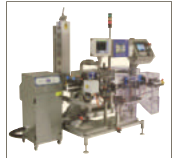
Coding and checkweighing: The Modified Garvens S2 machine
