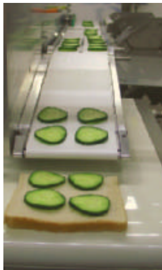
Sorting slices: CKF system delivers up to 120 items a minute for placing
