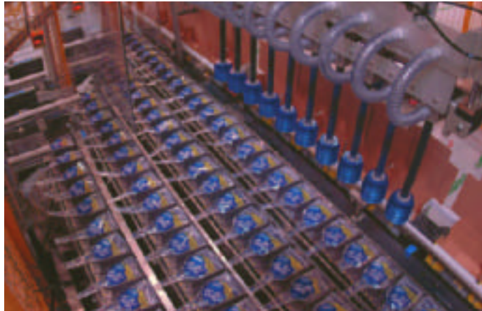
High speed case-packing: Langen robot cell at SipTop
