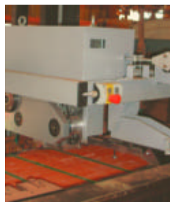
Faster strapping: Vario Master unit at Hanson's brick works
