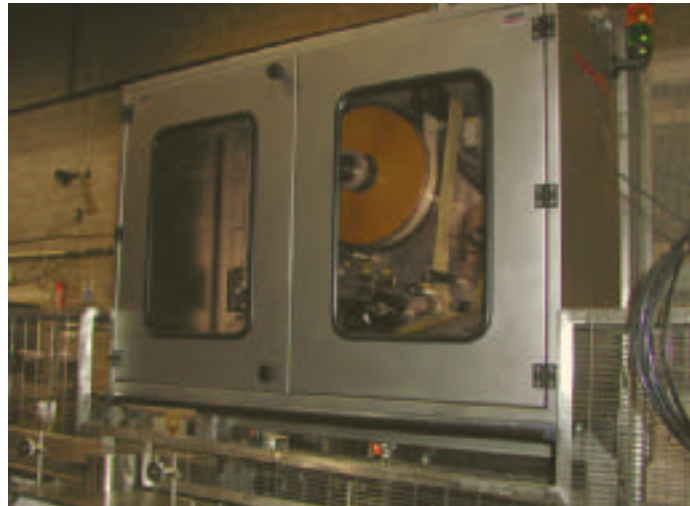
Enclosure-mounted: Logopak 515TK labeller is smaller than its predecessor
