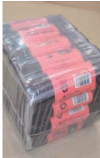
Double wrap system from MAF gives a low cost alternative to board. 10
