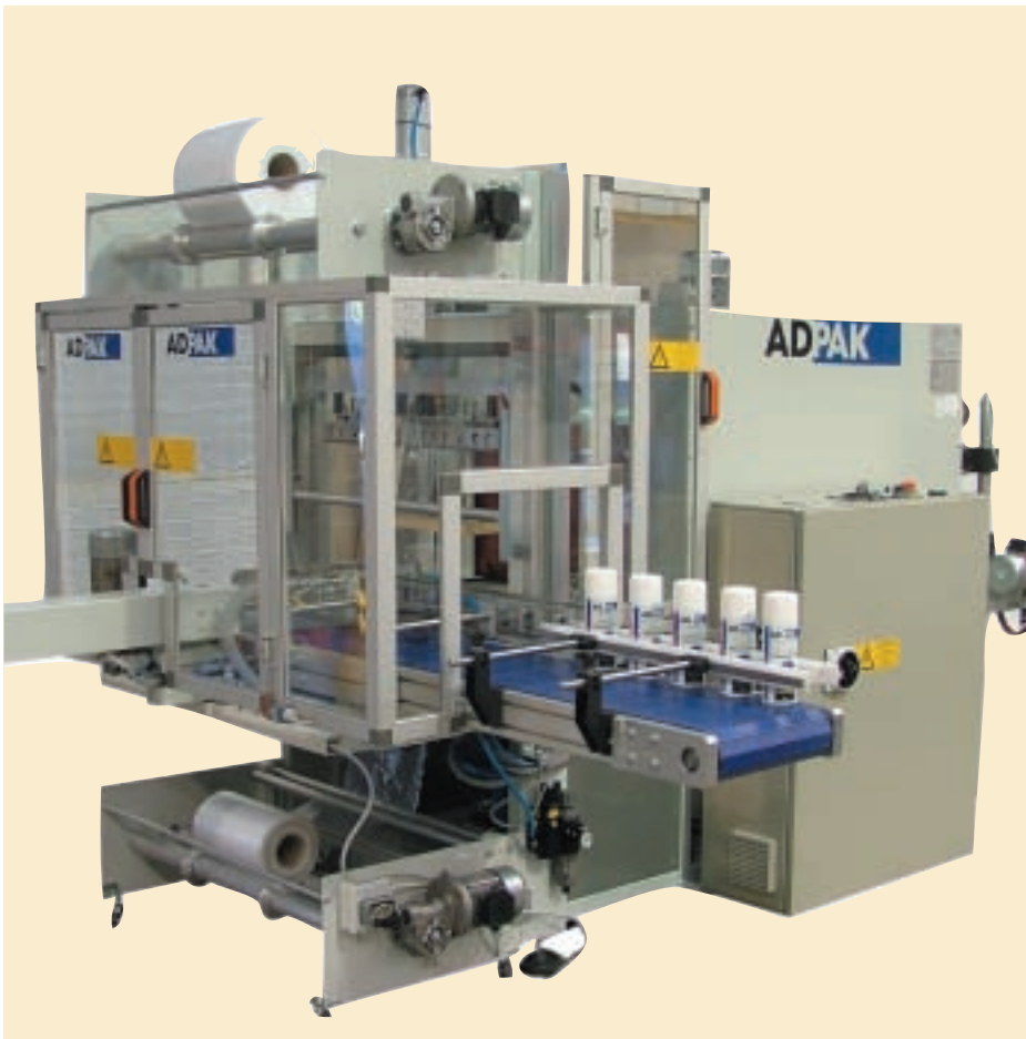
Sidefeed twin reel machine: Adpak 712 series can be equipped with automatic bottle collation
