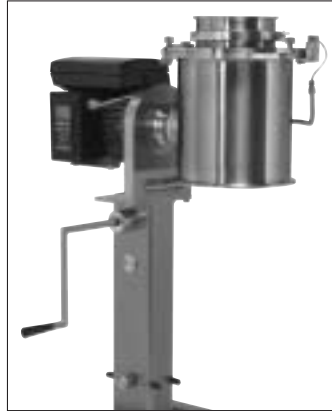
Sifting powders: Quadro Sifter pre-screening unit removes impurities
