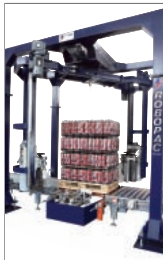
New twin arm pallet wrapper from Robopac can run at 170 an hour. 14
