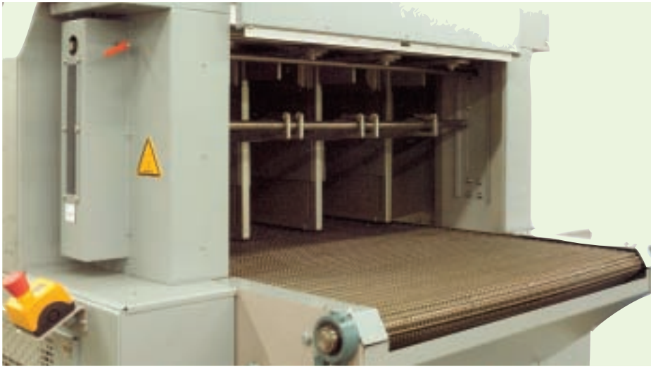
Air curtain: KHS system allows the shrink process to be monitored by a camera
