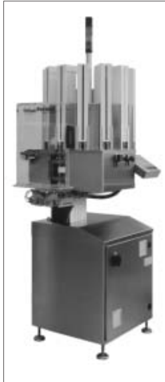
Automatic magazine: Revolver carries 16 trays of items for feeding
