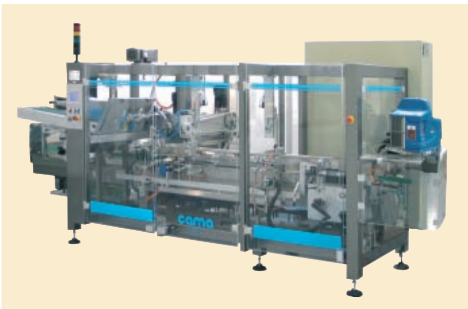
Barrel loader alternative: Cama has developed an overhead unit that saves space on cartoners
