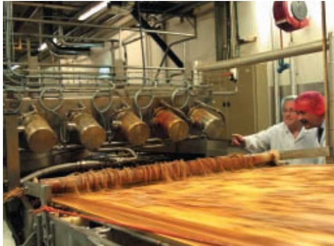
Clean-in-place: Twiglets line oil spinner motors no longer need removal
