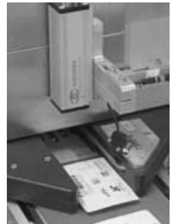
Inspecting the lidding: One of the cameras on the Scanware machine
