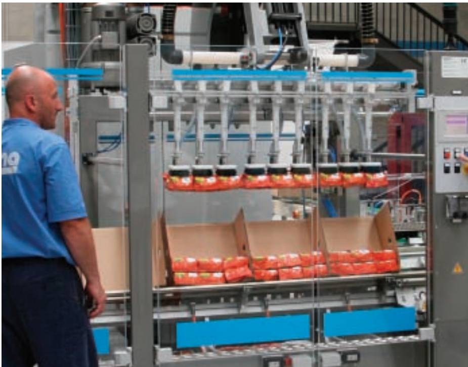
Loading block-bottom bags: Above: Robotic pick-and-place section. Below: The complete line
