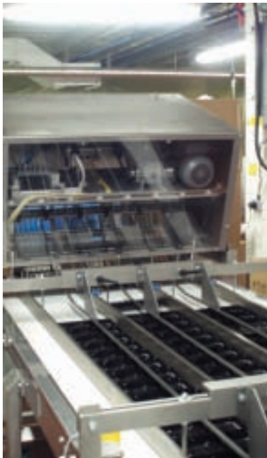
Three-lane denesting: Pneufeed unit delivers trays for chocolate fingers
