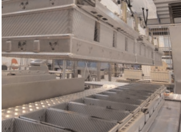
RTS Flexible Systems: Robotic bread tin handling for Warburtons
