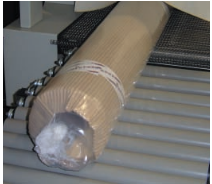
Side-feed wrapper: Panaz has automated the wrapping process for rolls of cloth
