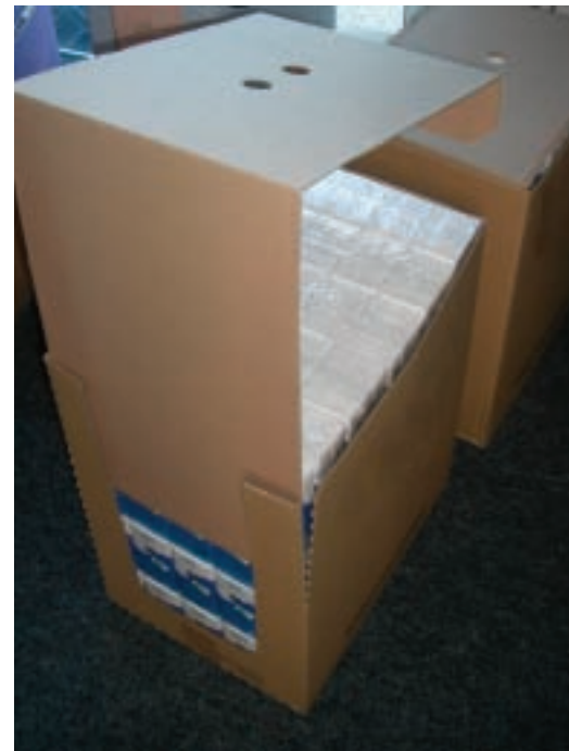
Side-loaded case: Tissue packs are loaded into this two-piece case on a Focke machine
