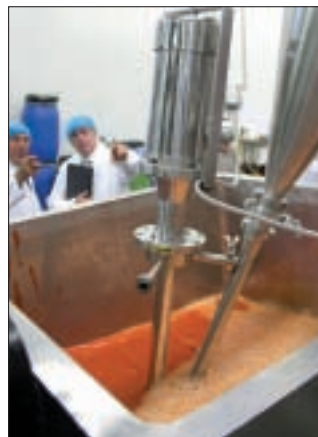
Ytron-Y ByPass high shear mixer employed on batches of fruit juice. 37
