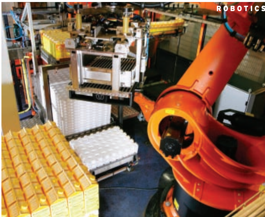
Juice merchandising: Kuka robot at Arla Foods in Sweden handles brik and gable top cartons
