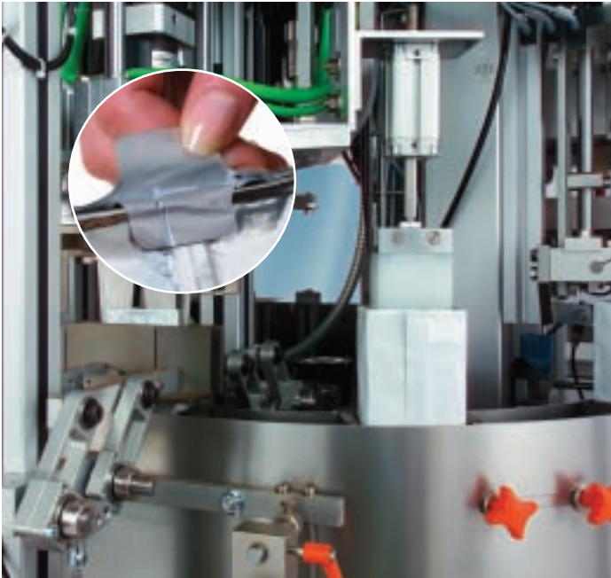
Choice of reclosure: Bosch filler with (inset) easy peel-open system
