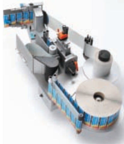
Labelling station: The Herma 400 Slim Line
