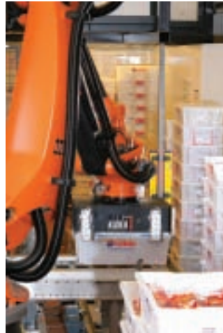
Order assembly for road transport using a Kuka robotic system. 11
