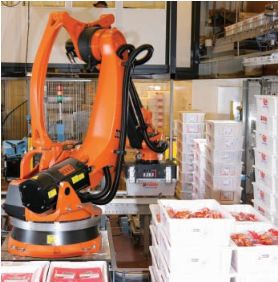
Order assembly: Kuka robot at Norwegian meat processor Gilde directs containers to lorry loading bays
