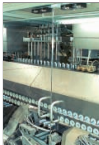
TFS 80-6 tube filler from Oyster-IWK is capable of 510 a minute. 25
