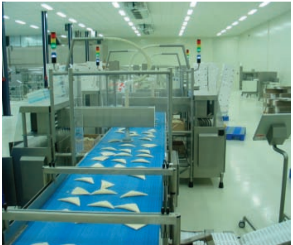
Linear drive: Roboxis T-robot uses linear drive and is aimed at the food industry
