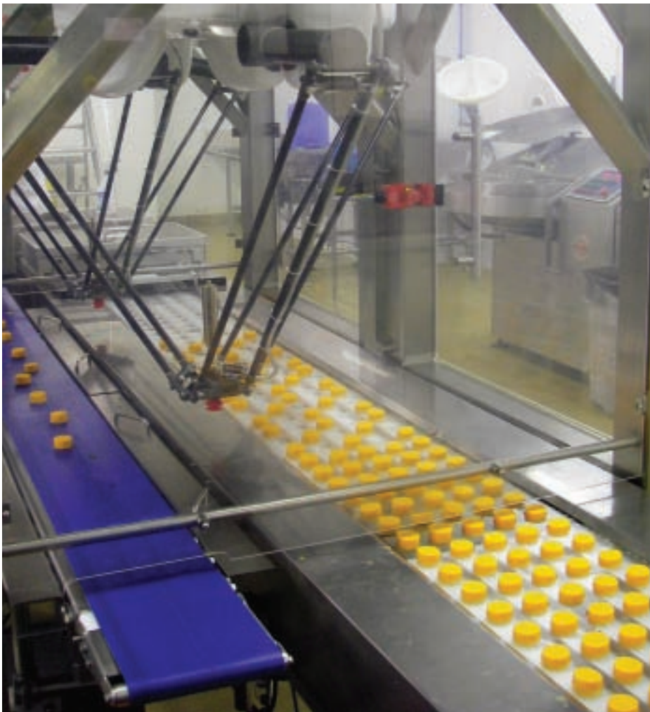
Reducing giveaway: RTS system at Ilchester Cheese measures portions as they are picked
