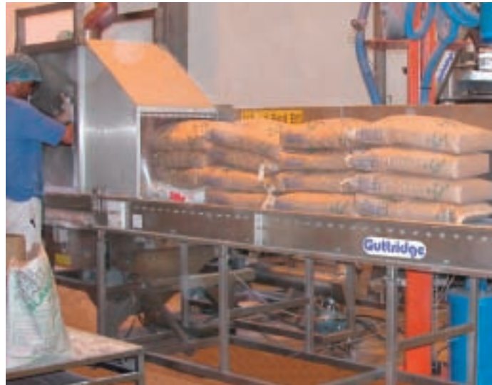
Raising powders: Guttridge system lifts ingredients to a height of 2.7 metres
