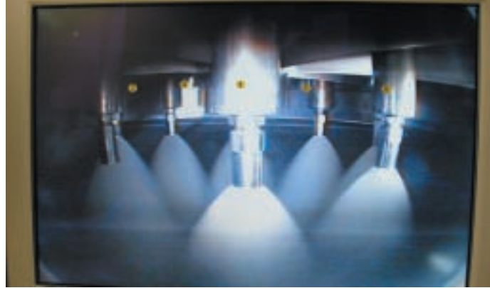
Cameras on spray nozzles: Niro's monitoring system in action
