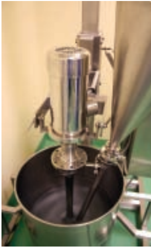
Ytron-Quadro's mixer for the production of solutions and suspensions used for film and sugar coated tablets
