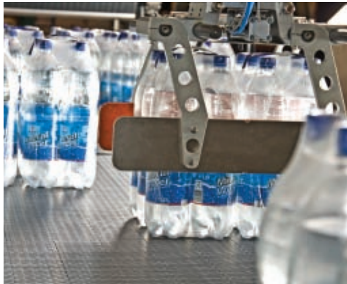
The Robobox pack grouping station from Krones
