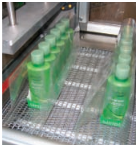
Adpak's side feed automatic shrink wrappers for Hallam Beauty
