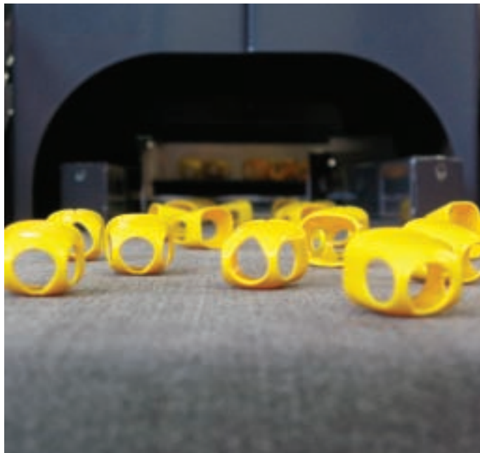
SVIA's flexible feeder and vision system for robot guidance ensure miniature plastic vests feed to the correct Tampoprint machine
