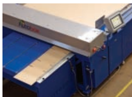
HIPAK ONE quick set corrugated box making machine
