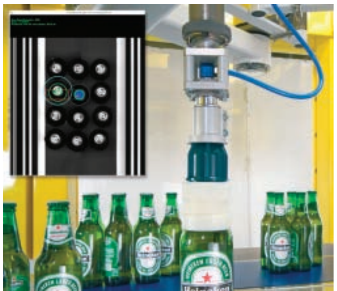
Scanners carry out a quality check in conjunction with the Schubert image processing system
