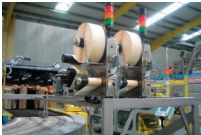
Cott Beverages has installed two purpose-built, gantry mounted Logopak print & apply machines
