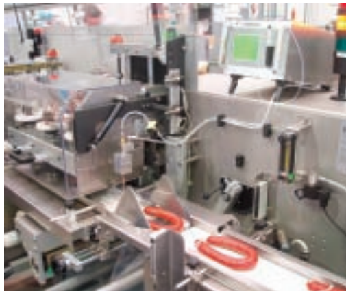
Synchropack's Pack 600, part of the Integrapak range, designed for MAP applications
